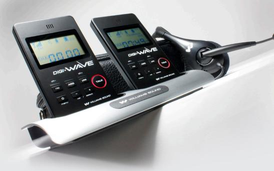
Ten DLT 100 digital transceivers were set up as a wireless intercom system, allowing the control room staff to communicate immediately and accurately in full-duplex mode with cameramen, lighting control, the audio engineer and the production manager in their different house locations. The control room staff spoke and operated as the central hub, while remote crew members participated as listen-only or by accessing two-way mode with the quick push of a button.
